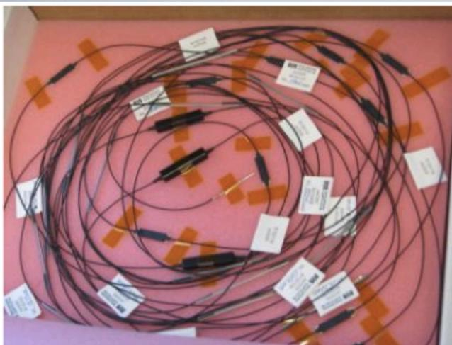
**Sensor array delivered to TPI assembled and ready for installation.**
